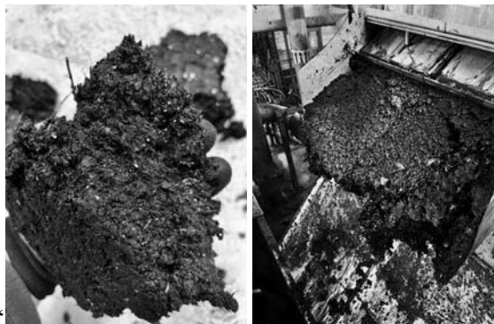
Figure 1 – Photo of dehydrated sludge after roller press
