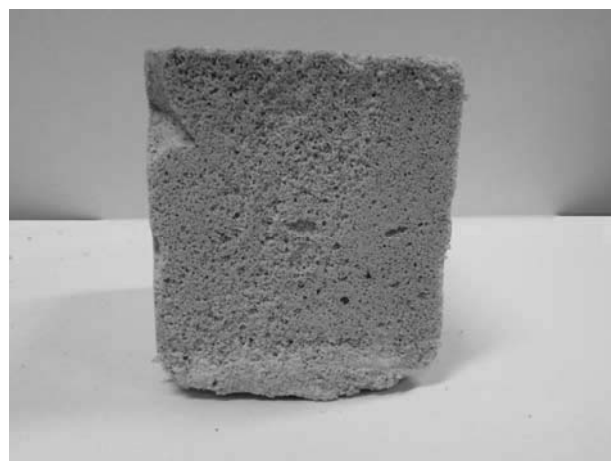
Figure 5 - Appearance of the sample on Zaturinsky bischofite and limestone aggregate
